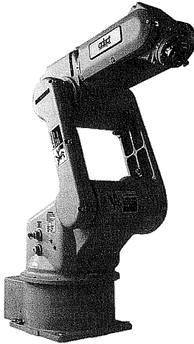
FIGURE 1.4: The Adept 6 manipulator has six rotational joints and is popular in many applications. Courtesy of Adept Technology, Inc.
