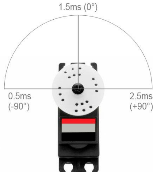
Hitec Standard Servo Showing Operating Angle vs Signal
